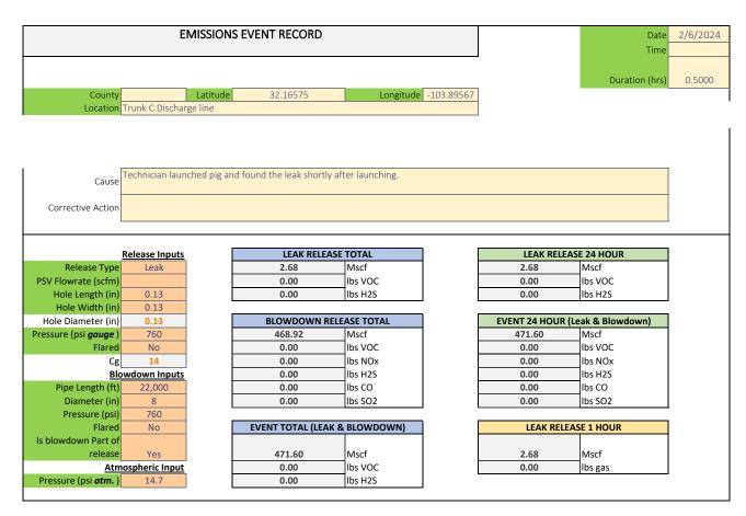
Volume of Gas Leaked (MSCF) = Diameter\*Diameter\*(Upstream Gauge Pressure + Atmospheric Pressure)\*Hours of Leak
