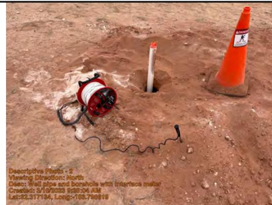
Well pipe and borehole with Interface meter
