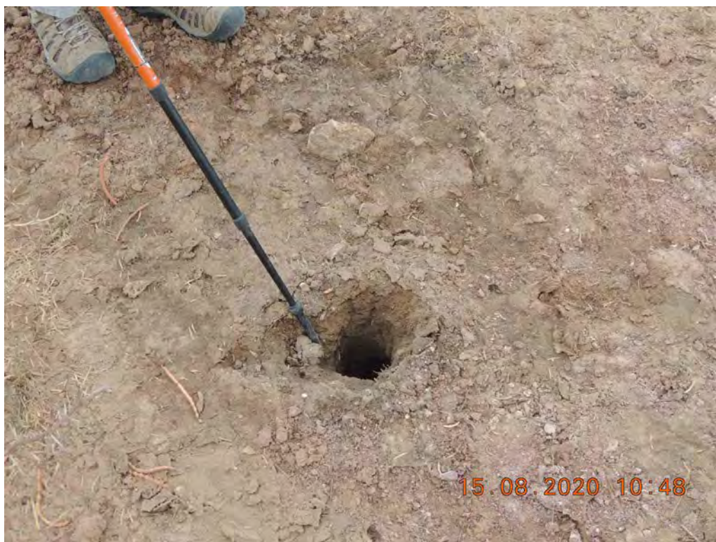
A 4" DIAMETER X 4+ FOOT DEEP HOLE DRILLED IN A SPILL AREA
