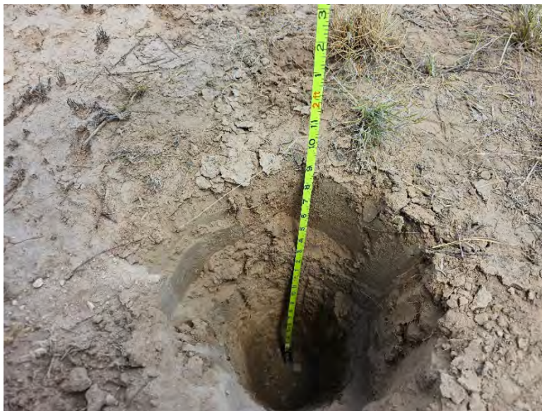
Figure 4: Lithology test hole, northwest corner of production pad. Date: 2023-08-30 13:31:09; GPS: 32.3893995, -103.1905543
