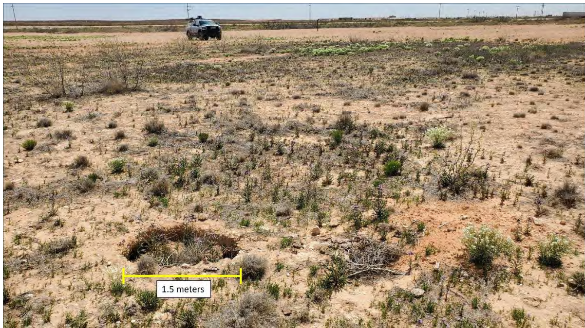
Figure 5: RKF 240423-D01: Example of a suffosion sinkhole. Please note that this image is of another similar feature in a similar orientation to a pad and is NOT RKF 240423-D01. Unfortunately, the photos taken during this survey were inadvertently deleted during downloading.
