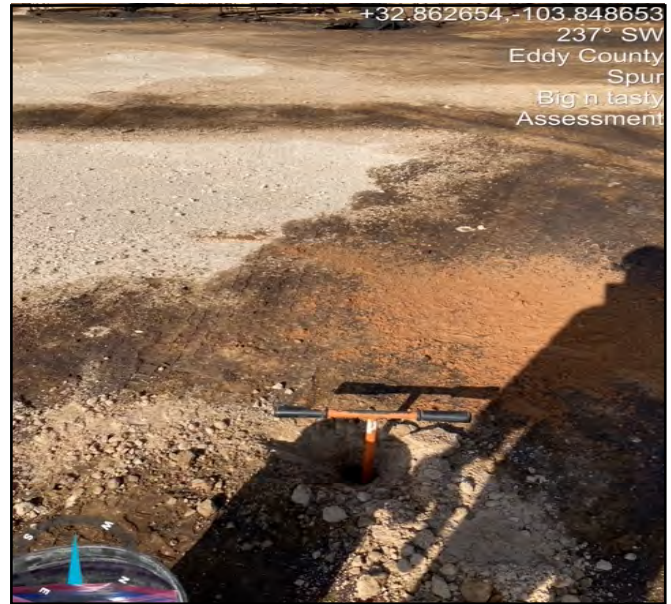
Photo of hand auger in ground to gather samples facing Southwest.
