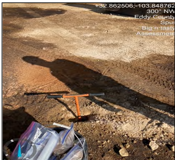
Photo of hand auger in ground to gather samples facing Northwest.
