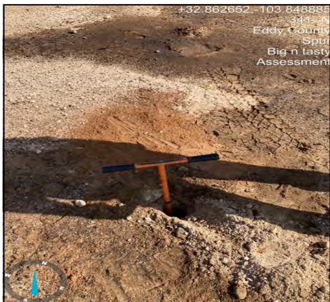
Photo of hand auger in ground to gather samples facing North.
