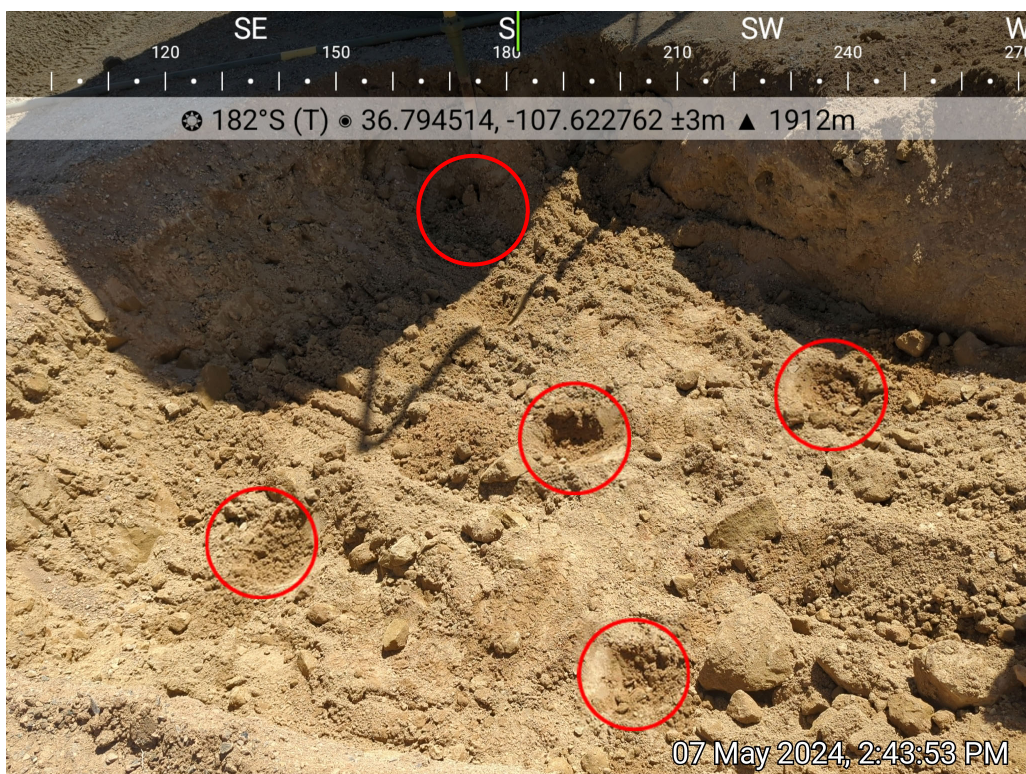
Photo 4: SS01 collected as a 5-point composite sample from the excavation area.
