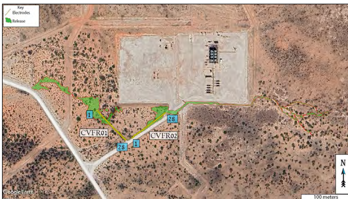
Figure 5: Survey overview. Two survey lines (denoted with white numbers) were conducted with 28 electrodes each at 3-meter spacing (yellow dots denoted with blue numbers). Background image credit: Google Earth. Image date: April 15, 2023. Image datum: WGS-84.
