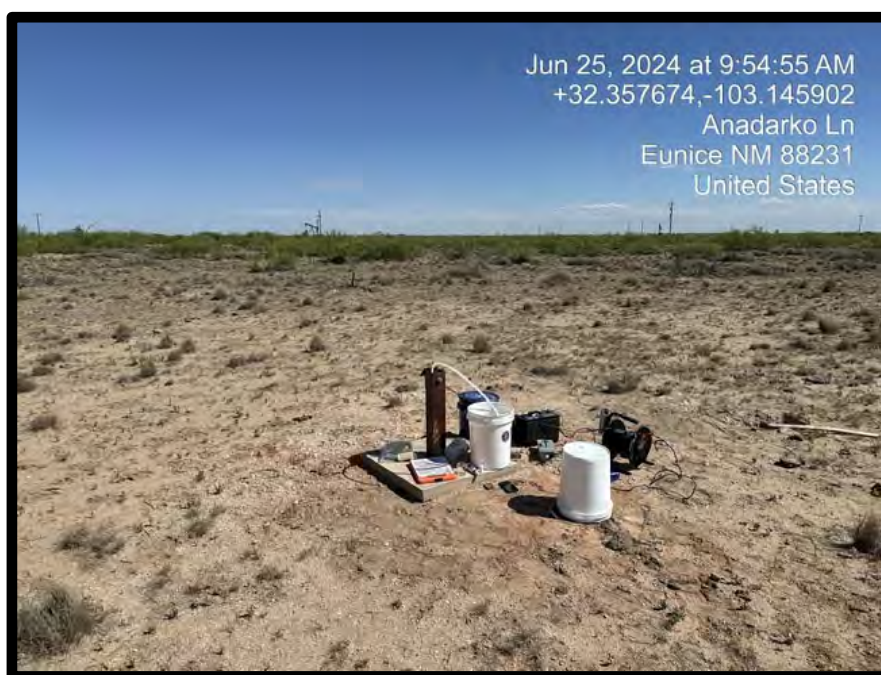
PHOTOGRAPH NO. 1 – A general view of the low-flow sampling methodology at monitor well MW-4 on June 25, 2024.
