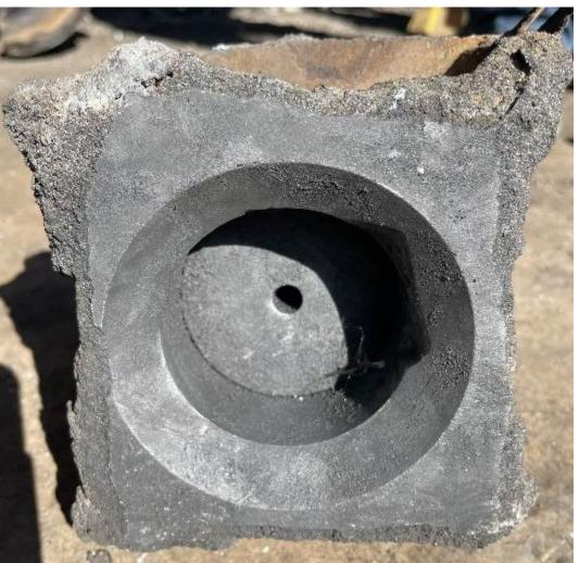
The center of the #2-cylinder head was blown out beyond the edge of the unit skid. A notch in the side of the center bore was due to contact with the piston retaining nut
