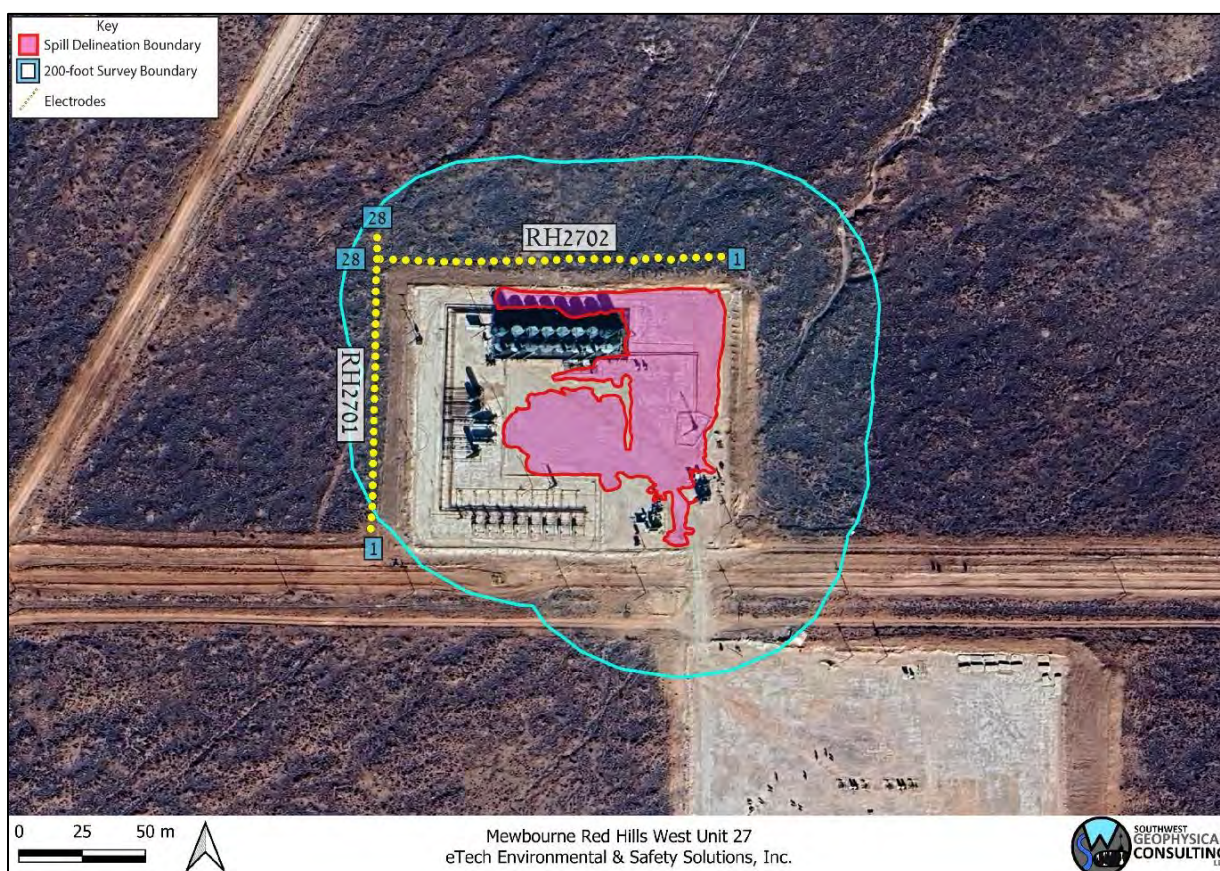
Figure 5: Geophysical survey overview. Both RH2701 and RH2702 were conducted with 28 electrodes each: all at 5-meter spacing (yellow dots denoted with blue numbers). Background image credit: Google Earth. Image date: December 12, 2023. Image datum: WGS-84.
