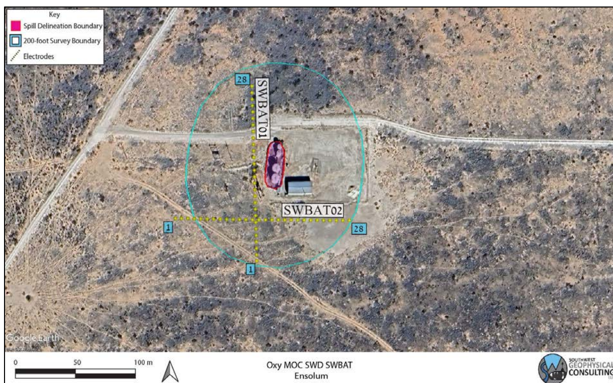
Figure 5: Geophysical survey overview. Two survey lines were conducted with 28 electrodes each at 5-meter spacing (yellow dots denoted with blue numbers). Background image credit: Google Earth. Image date: January 8, 2024. Image datum: WGS-84.
