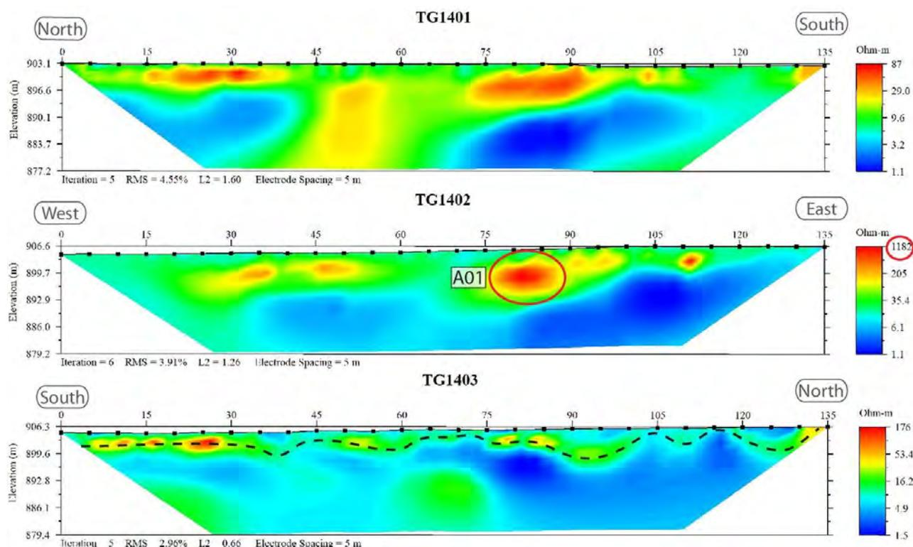
**Figure 8: 2D inverted resistivity sections. Red ellipse highlights high-resistivity anomaly. Black-dashed line indicates areas of possible instability. Reds and oranges indicate higher resistivity values. Yellows and greens are medium-resistivity values. Blues are low-resistivity values. Please note that the color scale is relative.**
