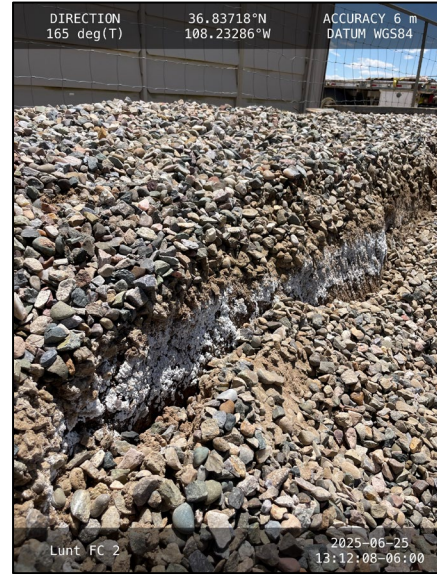
Photograph: 2 Date: 06/25/2025 Description: Impacted soil within secondary containment berm View: Southeast
