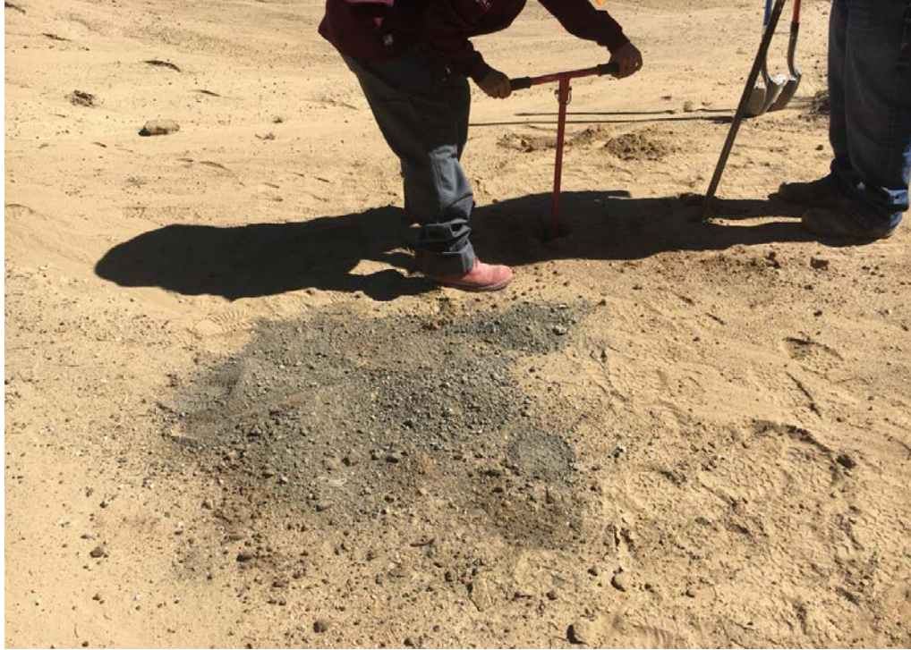
Photo 7. View of color change when auguring from loose sand into soft sandstone off pad. Photo taken September 25, 2025.
