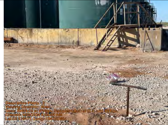
BH24-25 at 4ft bgs. Samples taken at 0, 2, and 4ft bgs.
