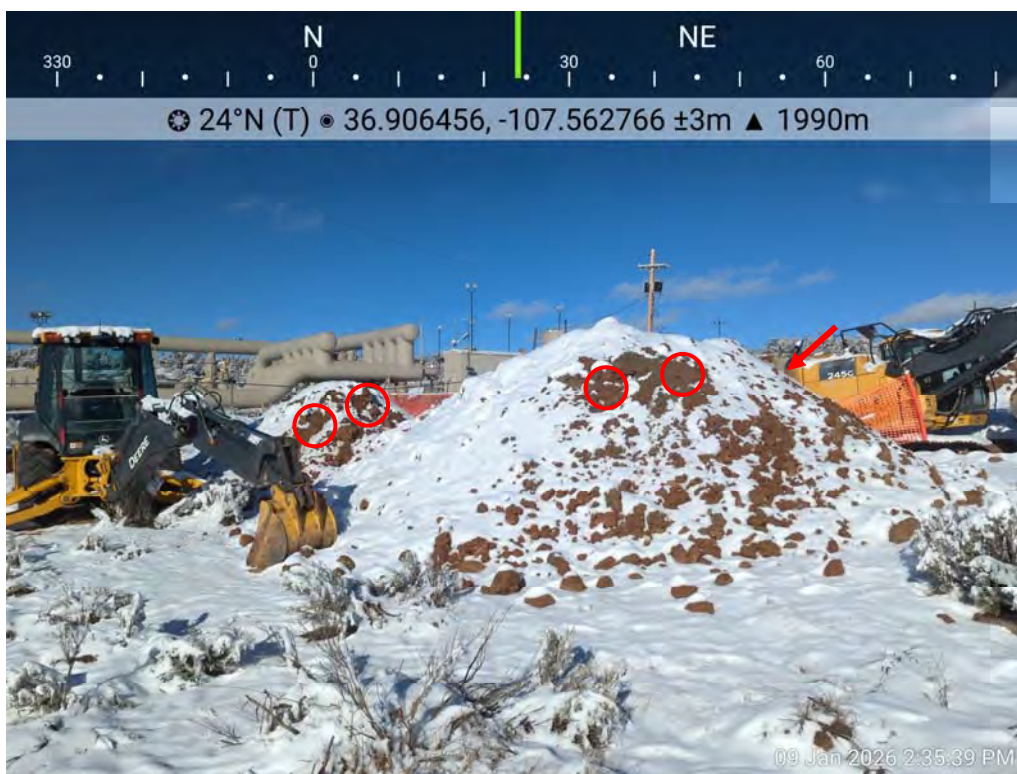
Photo 14: SS12 is a five-point composite sample collected from north spoils piles. Red arrow indicates sample point locations not visible in photograph.
