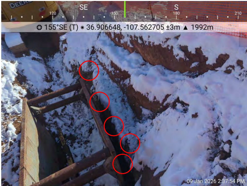
Photo 11: SS09 is a five-point composite sample collected from lower portion of west wall of excavation area.
