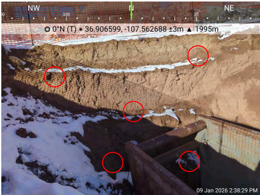
Photo 12: SS10 is a five-point composite sample collected from north wall of excavation area.
