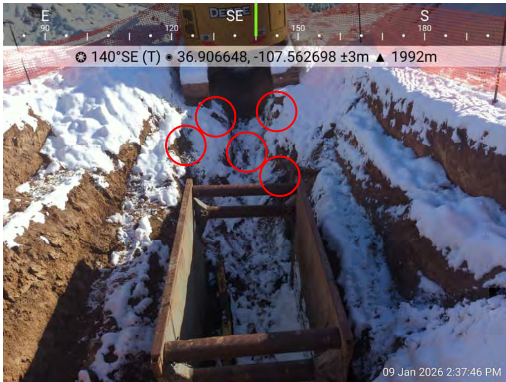
Photo 9: SS07 is a five-point composite sample collected from south wall of excavation area.
