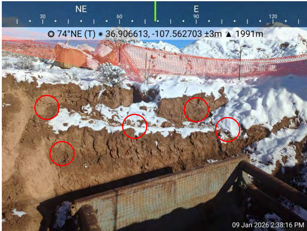
Photo 7: SS05 is a five-point composite sample collected from upper portion of east wall of excavation area.
