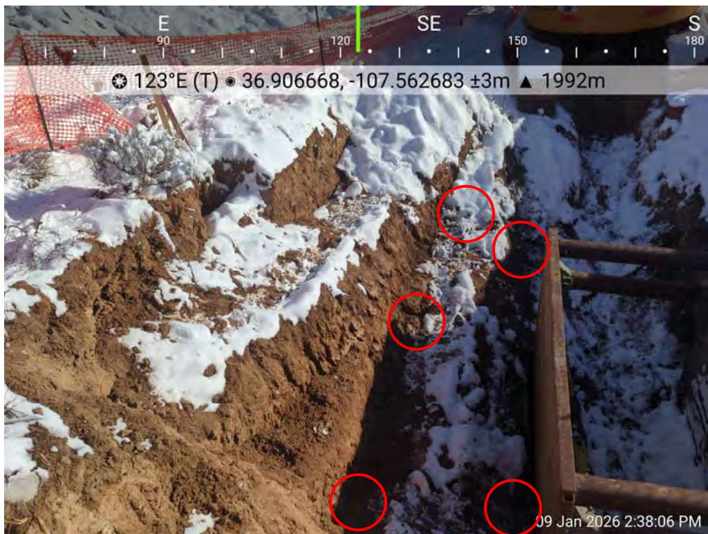
Photo 8: SS06 is a five-point composite sample collected from lower portion of east wall of excavation area.
