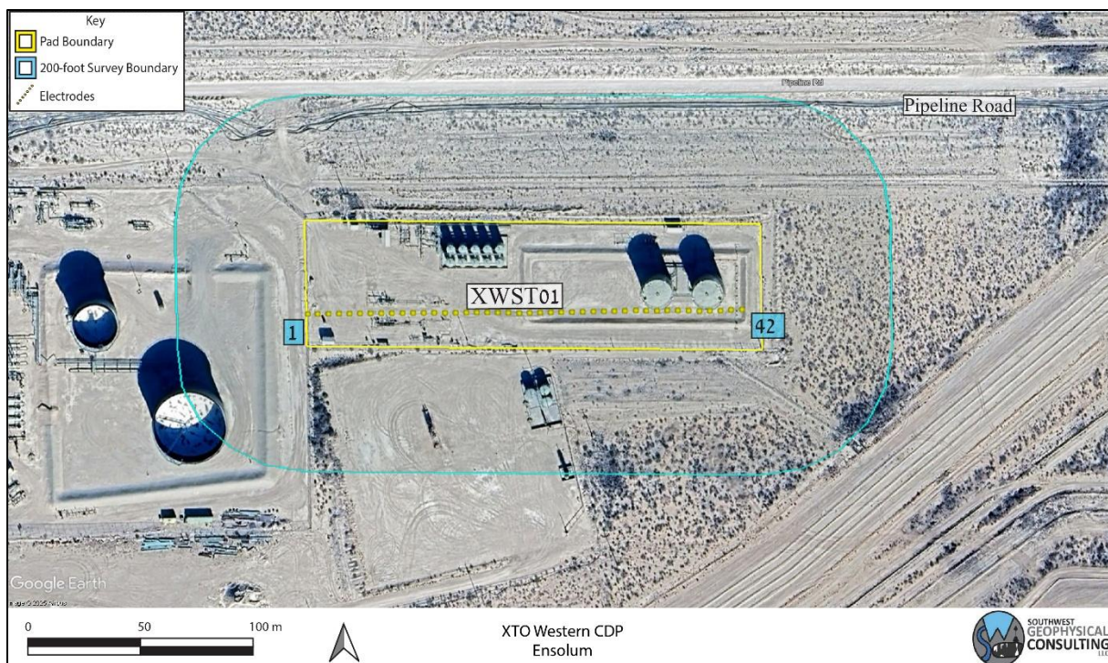
Figure 5: Geophysical survey overview. One survey line was conducted with 42 electrodes (yellow dots denoted with blue numbers). Background image credit: Google Earth. Image date: December 31, 2023. Datum: WGS-84.
