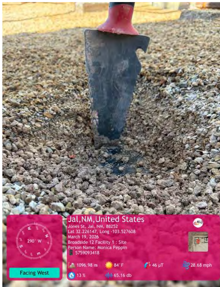
Depth of gravel with hand trowel.
