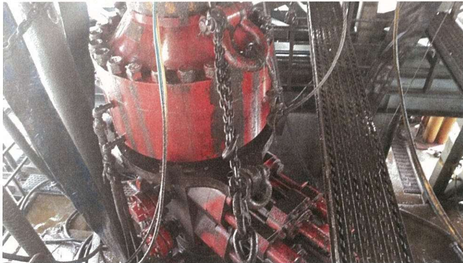
Figure 1: Winch System attached to BOP Stack
