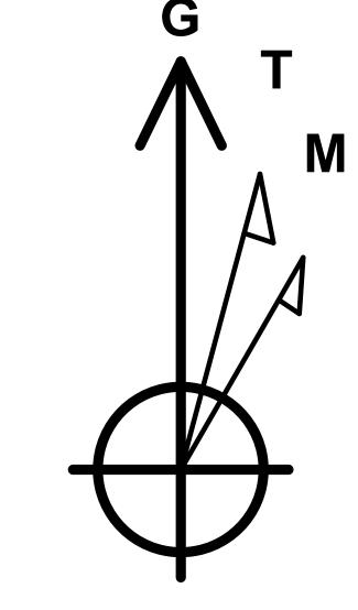
Azimuths to Grid North True North: 0.64° Magnetic North: 9.33°
