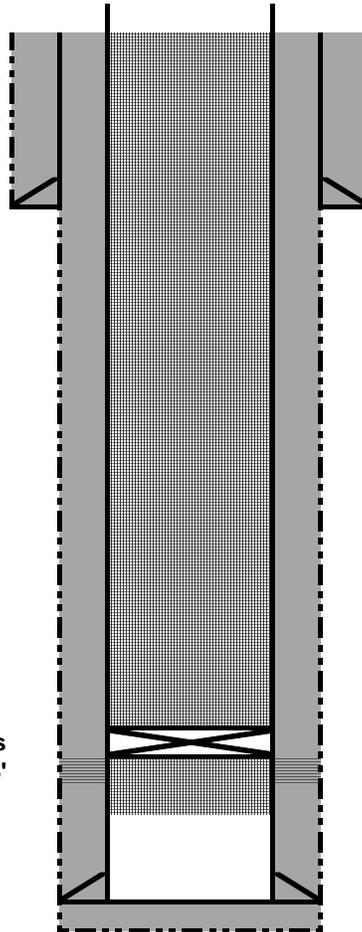
**Plug 2: From 1000' to surface, mix and pump Class G cement until cement circulation is seen at surface.**
