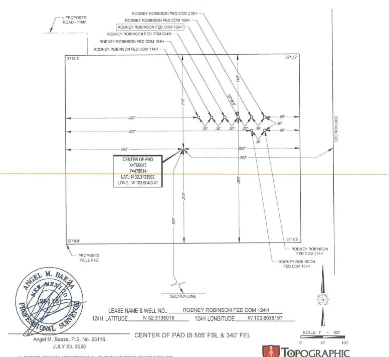
ALL BEARINGS, DISTANCES, AND COORDINATE VALUES CONTAINED HEREON ARE GRID BASED UPON THE NEW MEXICO COORDINATE SYSTEM OF 1993, EAST ZONE, U.S. SURVEY FEET.ELEVATIONS USED ARE NAVD88, OBTAINED THROUGH AN OPUS SOLUTION.
