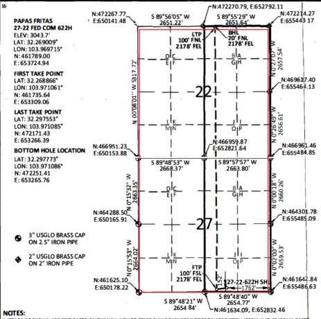
BEARINGS SHOWN ARE GRID BASED ON THE NEW MEXICO STATE PLANE EAST ZONE COORDINATE SYSTEM (3001), NAD 83 (2011), BASEQ FROM GPS OBSERVATIONS, OCCUPYING A WHS CONTROL POINT (5/8" REBAR), LOCATED AT NORTH: 456034.443, EAST: 653560.641, ELEVATION: 3101.373, DETERMINED BY AN OPUS SOLUTION ON DECEMBER 3RD, 2018.
