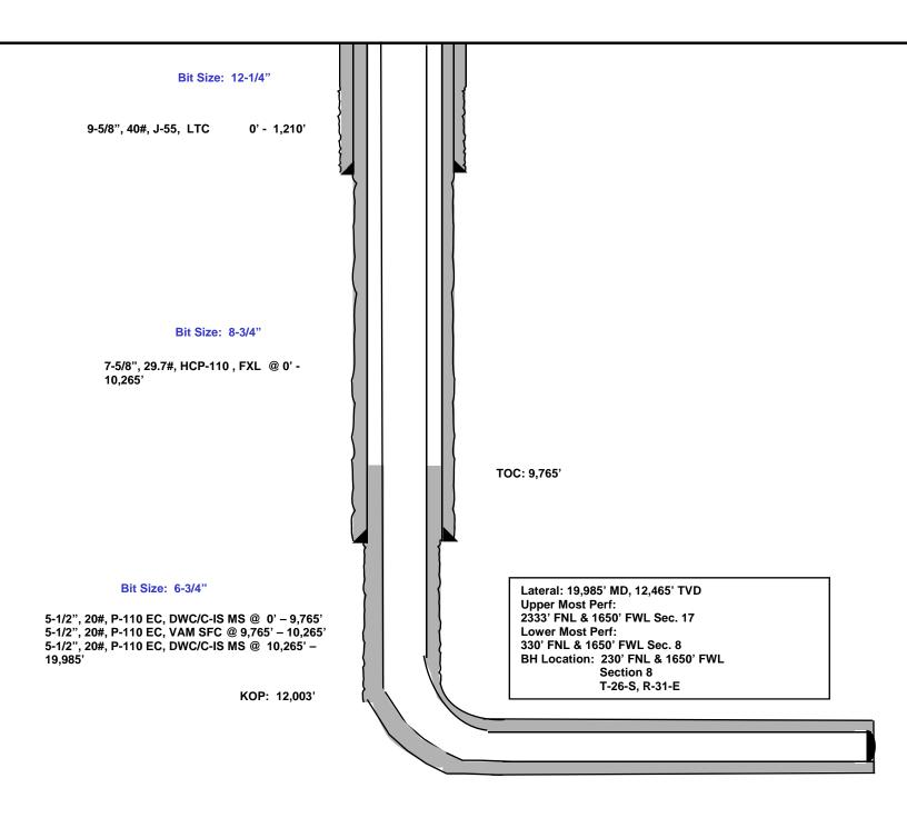
2230' FNL 1731' FWL Section 17 T-26-S, R-31-E Proposed Wellbore Design B GL: 3,272' GL: 3,247'
