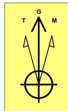
**Azimuths to Grid North** True North: -0.33° Magnetic North: 6.38° **Magnetic Field** Strength: 47501.0nT Dip Angle: 59.80° Date: 7/16/2020 Model: IGRF2020
