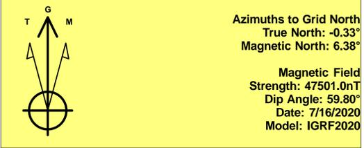
To convert a Magnetic Direction to a Grid Direction, Add 6.38°
