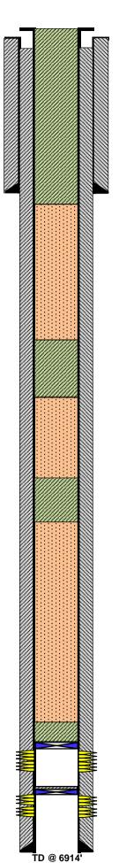
4. PUH & spotted 120 sx Class "C" cmt from 1139' to surf, RDMO, cut off WH, install dry hole marker, clean location, P&A complete. (Surf Shoe, Rustler, Water Board, & Surf Plug)
