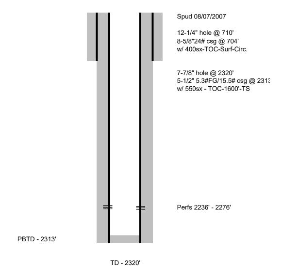
OXY USA Inc. - Proposed Bravo Dome CO2 Gas Unit # 101 API No. 30-021-20397
