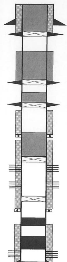
Perforate @ 286'. CR @ 265'. Plug IV: Circulate cement to surface w/ 23 sks Class G cement (26.5 cu.ft), 265'-0' Surface plug.
