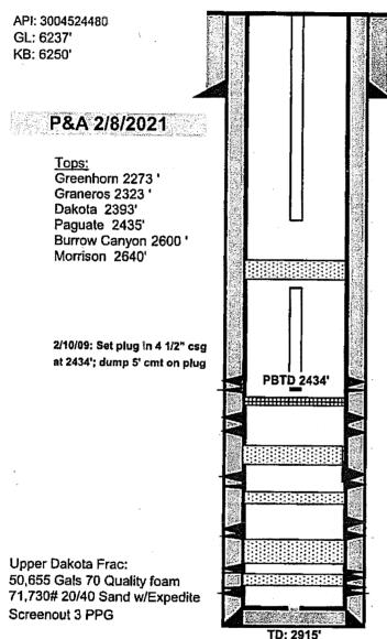
CUT OFF WELLHEAD. TOP OFF CMT W/30 SX. PUT DRY HOLE MARKER ON.
