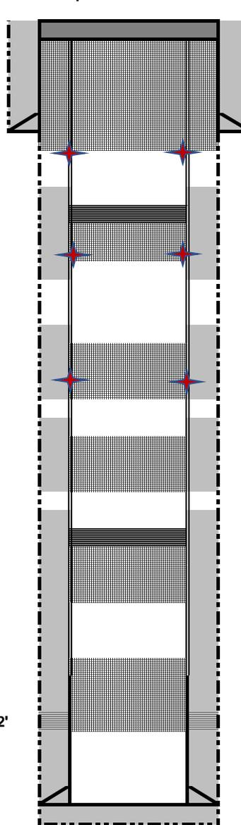
8-12-2021: Install P&A marker. Top off casing and cellar with 15 sx cement.
