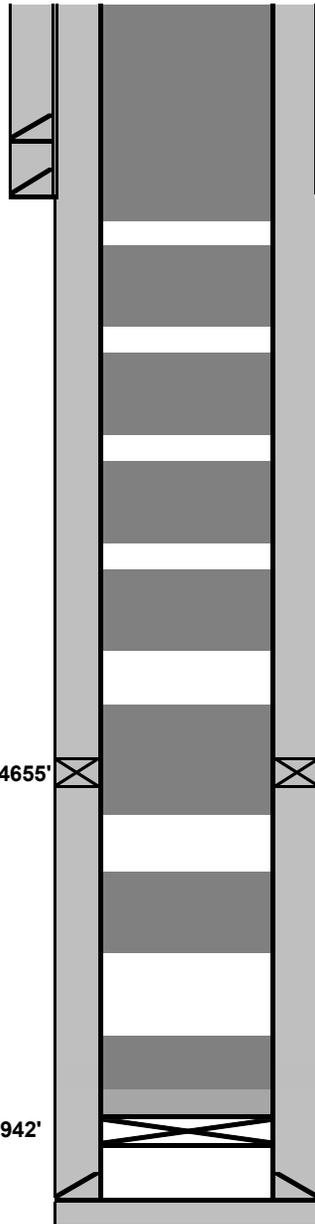
Plug 8: Surface casing shoe: Spot balanced plug from 512' to surface inside 4-1/2" casing.
