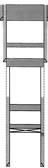
6. Perf'd 8 5/8" csg @ 375'. ND BOP & 8 5/8" well head. Pressured up on perfs to 1200 PSI. Dug out cellar & cut off anchors & well head. Spotted 125 sx class C cmt @ 425' & circulated to surface.
