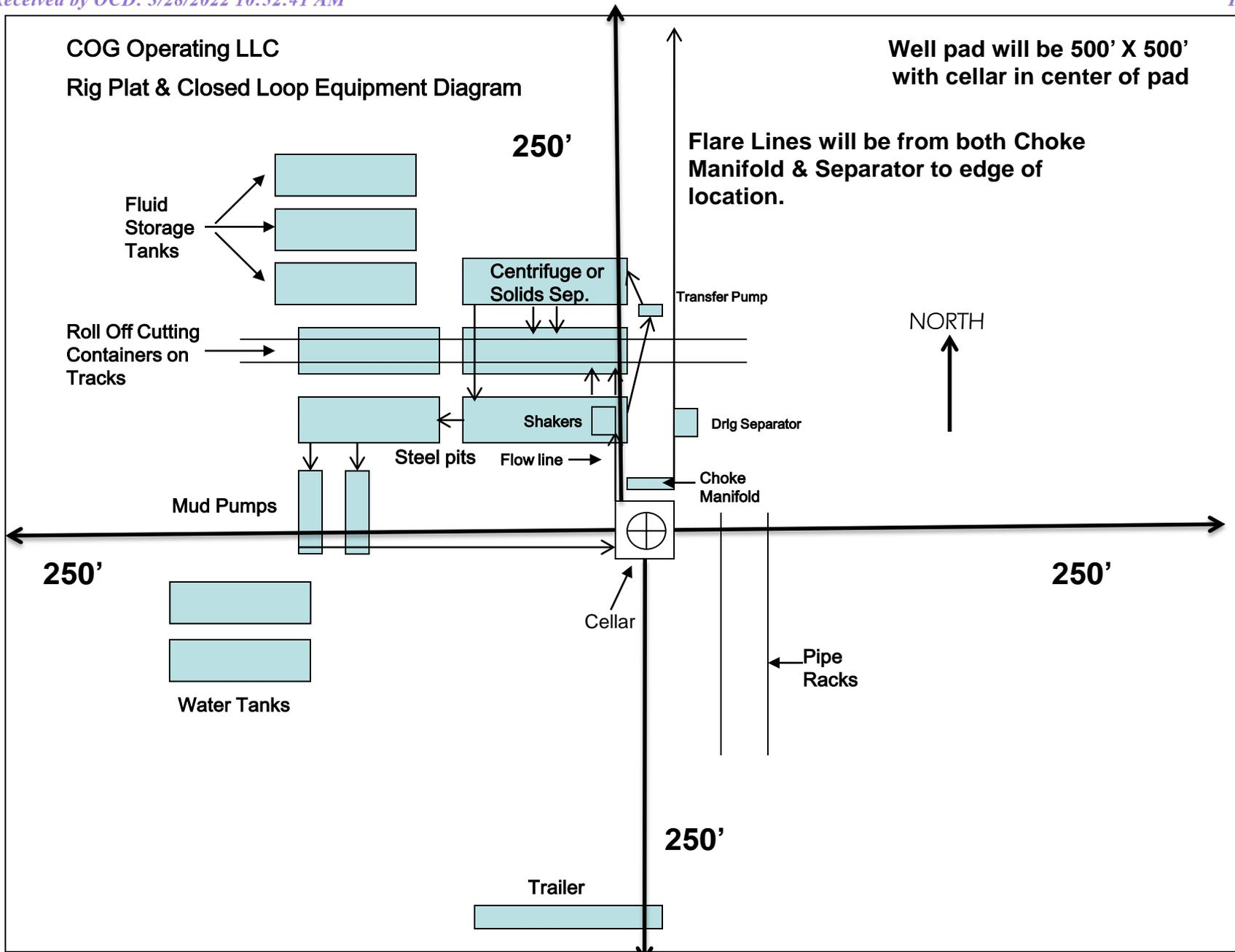
Flare Lines will be from both Choke Manifold & Separator to edge of location.
