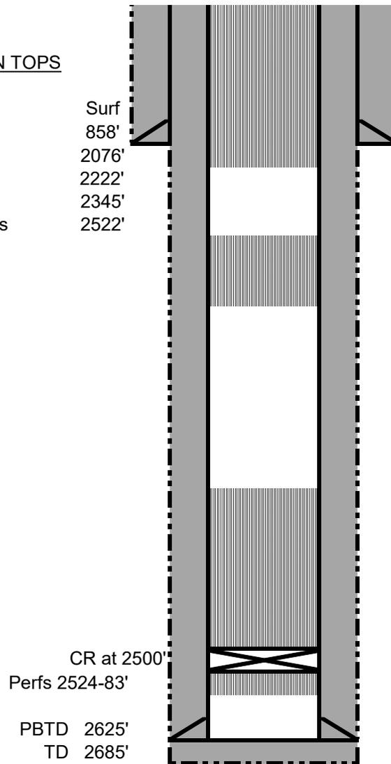
Plug 4: Surface shoe and surface plug: Spot balanced plug from 179' to surface.
