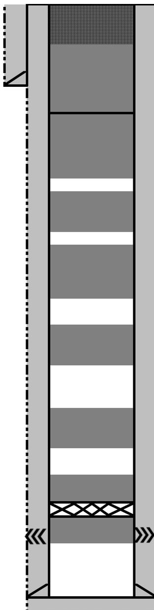
2-12-2022: Cut off WH. TOCs at 58' and 68'. Install P&A marker. Top off casing, annulus and cellar with 56 sx.
