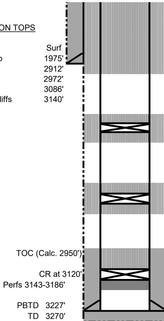
Plug 3: Surface shoe and surface plug: Perf holes at 152'. Tie onto 4-1/2" casing and mix and pump sufficient cement to bring TOC to surface, inside and outside.
