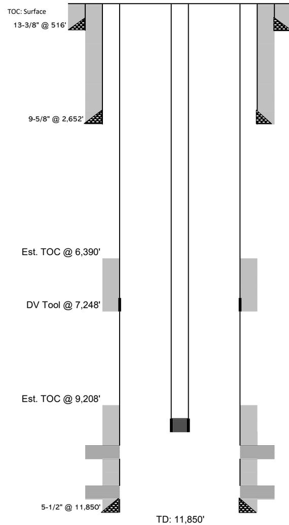
8/15/14: Hung tubing on wrap around tubing head & dropped 5/8" x 6' cold rolled steel bar in tubing
