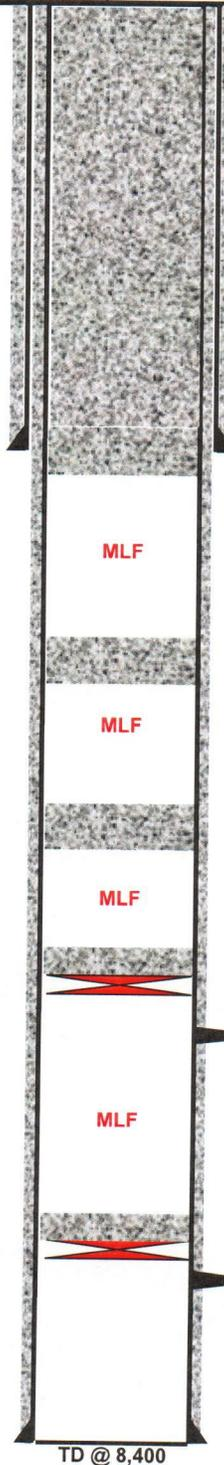
Spot plug @ 1570' to surface, 155 sx class C. WOC and Tag. (Top of Salt & Casing Shoe).
