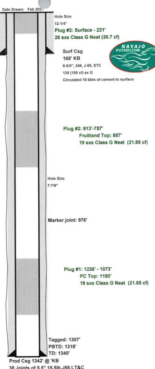
38 Joints of 5.5",15.5lb,J55 LT&C CMT: LEAD: 160SX(308.8cf) 35% POZ, TAIL: 115SX(132.2cf) CIRC 12BBL CMT (38SX) to surface
