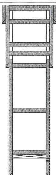
7. PerPd csg @ 150'. Sqz'd 100 sx class C cmt @ 150' & circulated to surface on 8 5/8" & 13 3/8" csg.
