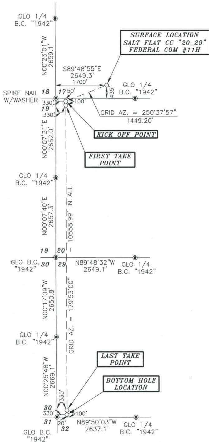
Basis of Bearings - GPS Geodetic Measurements
