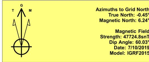
To convert a Magnetic Direction to a Grid Direction, Add 6.24°
