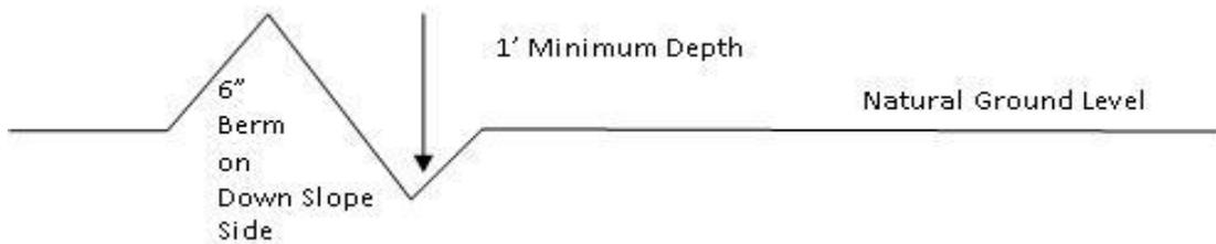
All lead-off ditches shall be graded to drain water with a 1 percent minimum to 3 percent maximum ditch slope. The spacing interval are variable for lead-off ditches and shall be
