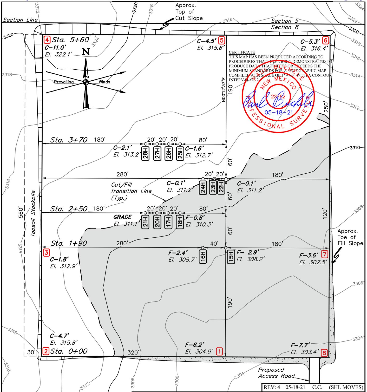
NOTE: Earthwork Calculations Require a Fill @ some of the Location Stakes For Balance. All Fill is to be Compacted to a Minimum of 95% of the Maximum Dry Density Obtained by AASHTO Method t-99.
