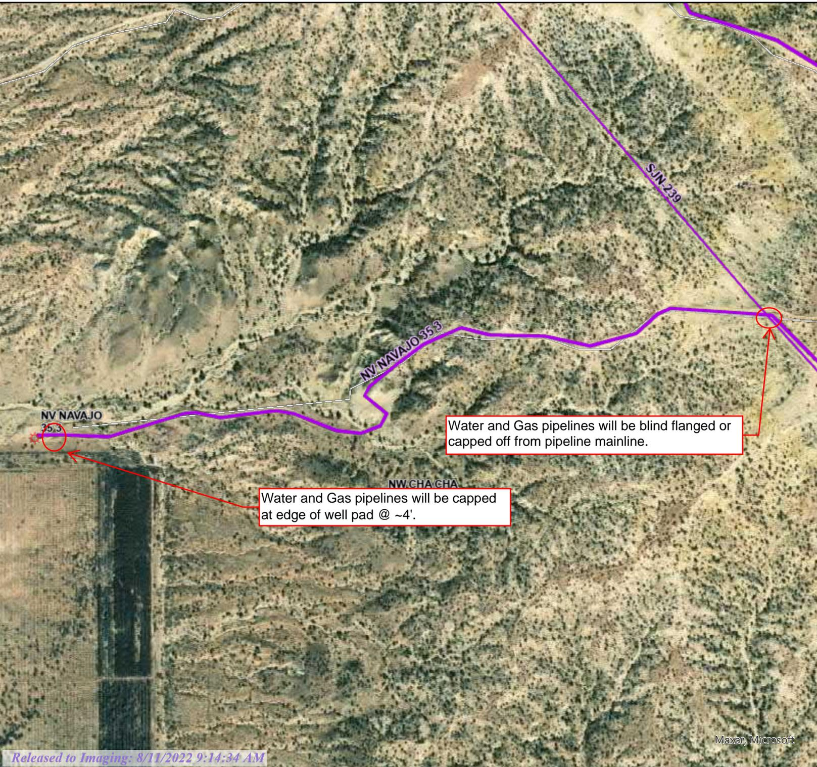
Water and Gas pipelines will be blind flanged or capped off from pipeline mainline.
