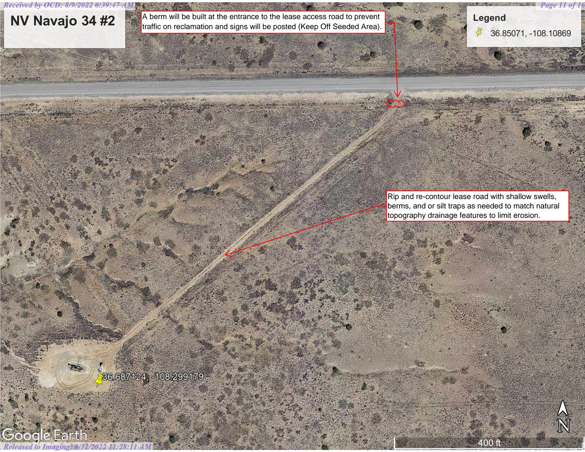
Rip and re-contour lease road with shallow swells, berms, and or silt traps as needed to match natural topography drainage features to limit erosion.
