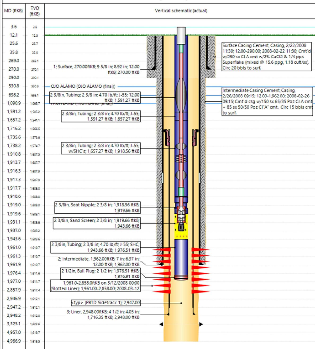
Surface Casing Cement, Casing, 2/22/2008 11:30; 12.00-290.00; 2008-02-22 11:30; Cmt'd w/250 sx CI A cmt w/2% CaCl2 & 1/4 pps Superflake (mixed @ 15.6 ppg, 1.18 cuft/sx). Circ 20 bbls to surf.
