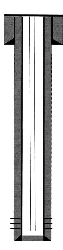
8-5/8" 24# J-55 casing @ 138'. Cemented with 100 sks Class B cement w/2% CaCl2 . Circulated cement to surface. Hole size 12  $\frac{1}{4}$ ".
