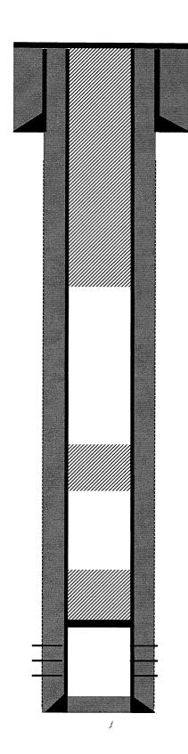
8-5/8" 24# J-55 casing @ 138'. Cemented with 100 sks Class B cement w/2% CaCl2 . Circulated cement to surface. Hole size 12  $\frac{1}{4}$ ".
